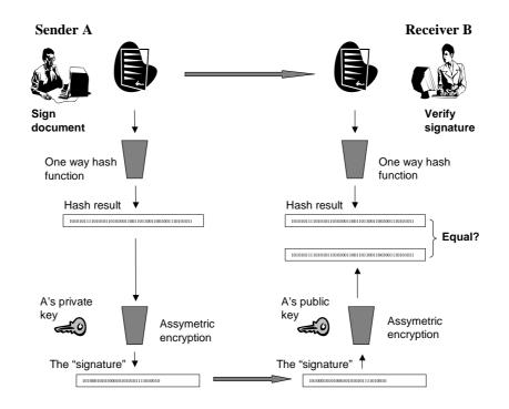
Figure 1: The digital signature process
